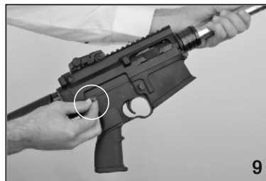
9) Remove the takedown pin with a tool to separate the receivers.
