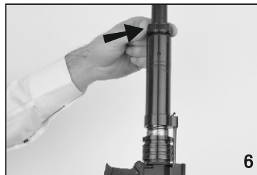
6) Remove the piston nut to anti-clockwise side.
