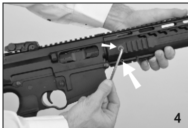
4) Remove the allens screw with 4-3 number allen key on the handguard.
