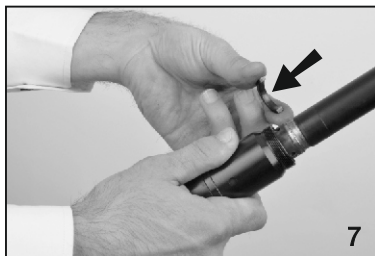
7) While holding gas chamber back side, remove the gas chamber's oring. (55)
