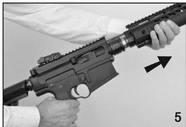
5) Remove the handguard towards arrow way.
